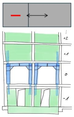
while the central column is loaded in compression only. This structural concept enabled the efficient design of the strip foundation as a two-span beam.
